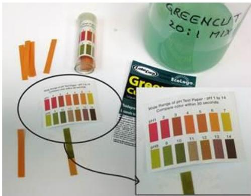
1. **Check the pH regularly of the bath/table** in order to maintain a 20:1 Water/GreenCut ratio by using pH test strips to do a color match; **pH should be between 9 and 10** for optimum performance.
