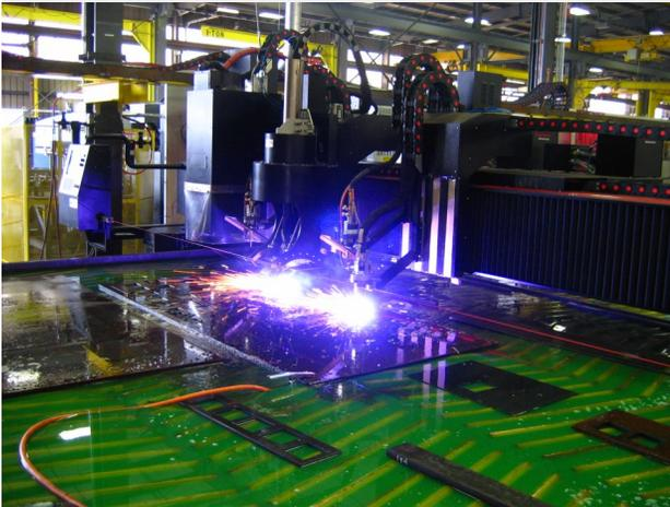
Plasma Arc Cutting removes metal by using a constricted arc to melt a localized workpiece, and removing the molten material with a high-velocity jet of ionized gas from the orifice. Plasma Arcs operate at 10,000°C -14,000°C (18,000°F -25,000°F).
