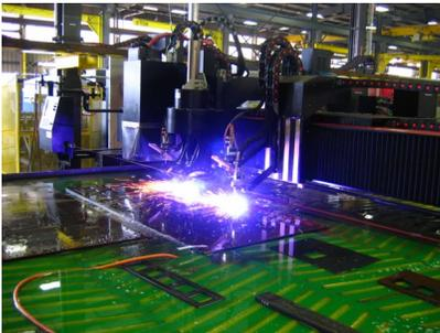
**Oregon Iron Works**, a pioneering structural fabricator from Oregon has been using LubeCorp's GreenCut Plasma Arc Water Table Fluid since the year 2007 to treat a large CNC plasma cutting system with a 15,000 gallon water table in its Vancouver, WA facility. Plasma water table technology is often chosen by large industrial manufacturers, such as bridge fabrication companies, due to design limitations and cost of the HVAC units needed to evacuate large down-draft tables.
